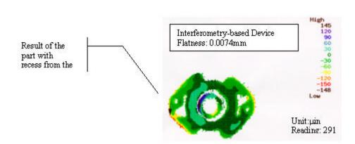
The part with a recess was later measured by another grazing-incidence interferometric device owned by a major automotive part supplier. As shown in the picture (below), the interferometric device did not only fail to detect the recess, build also created its own version of the surface (as a protrusion). Again, the reading (0.0069 mm) is not even close to the amount of recess (missed by 7 folds).
